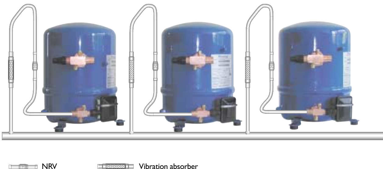
Figure 3.6 Discharge header below compressor discharge connections.
