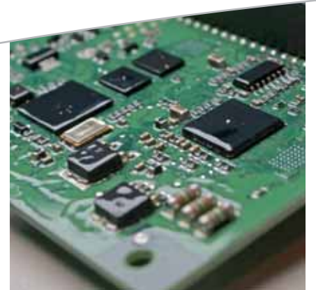
Coated control boards are available for harsh environments.
