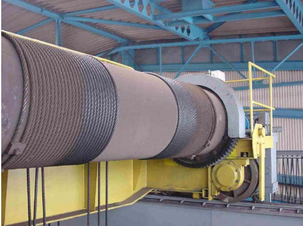
Fig. 2. The common shaft is driven on the both sides. The visible lines keep the hook.
