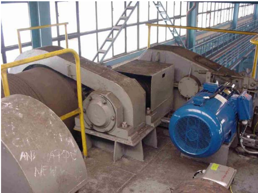
Fig. 3. The motor 18.5kW drives one side of the common shaft. Two drive ratio stages are visible. An identical system is situated on the other side of the shaft.
