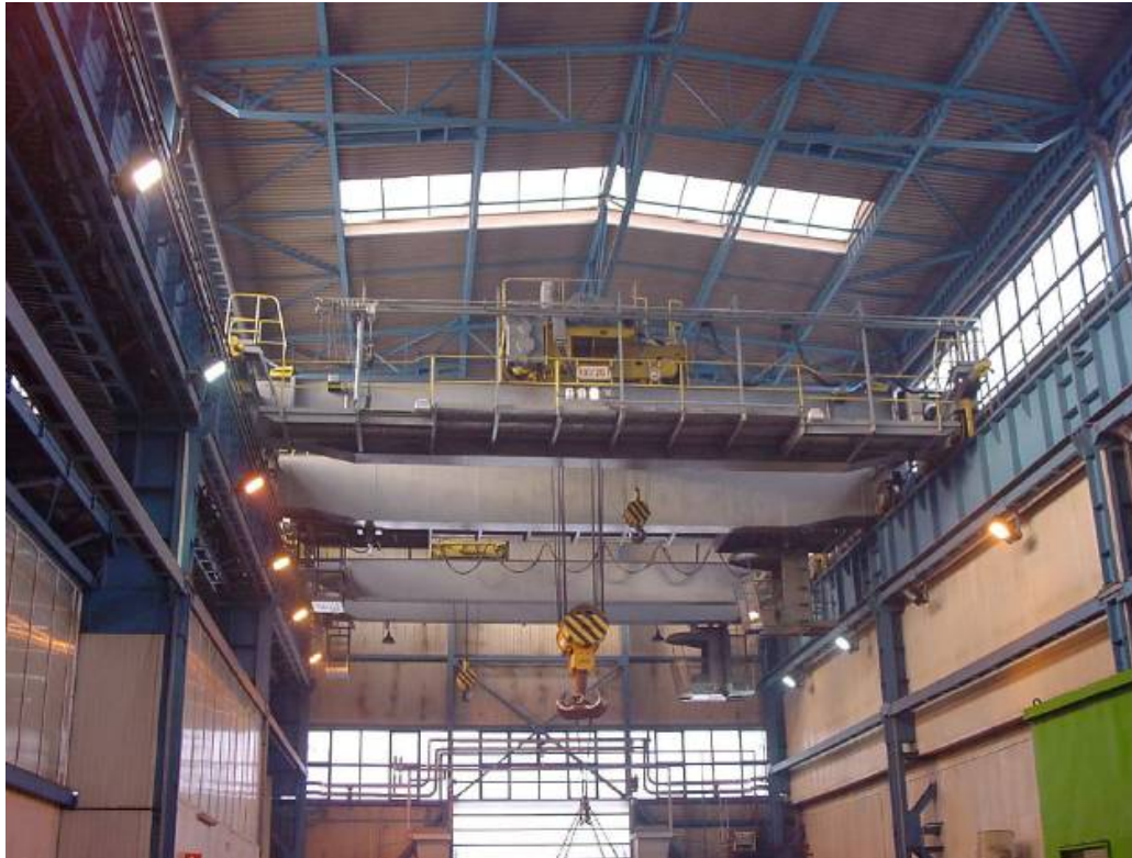
Fig. 1. The overhead travelling crane being the subject of the modernisation. The photograph presents the hook of the main hoisting winch (bigger) and of the auxiliary hoisting winch (smaller).
