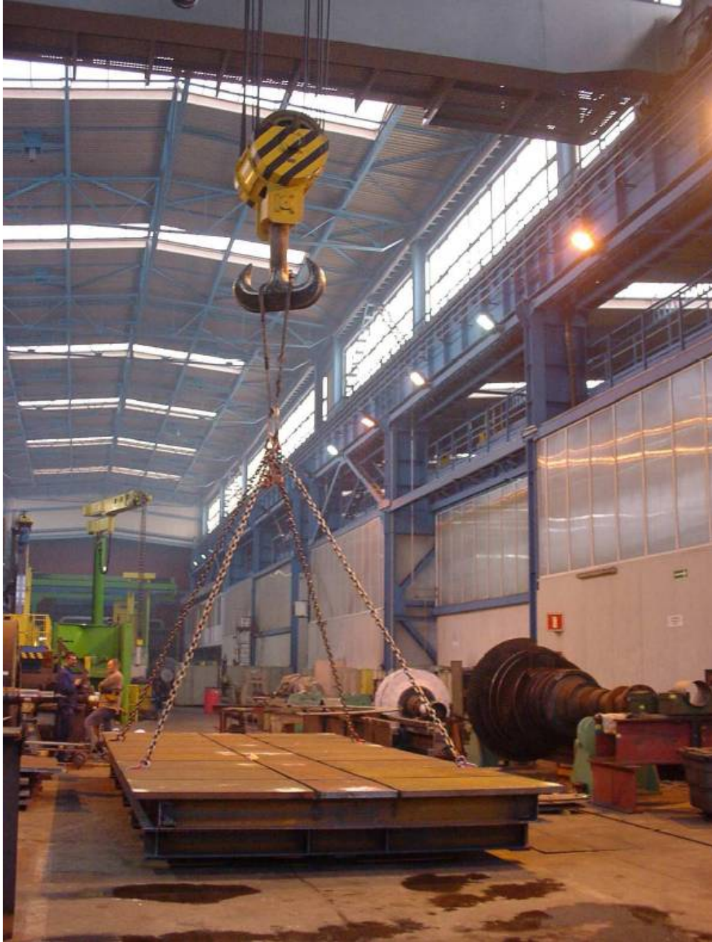
Fig. 5. The hoisting winch during the 20t load test.
