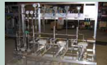
Skid systems: Daisy-chain pumps for increased capacity, or design one-skid arrays for chemical injection, condensate transfer, etc.
