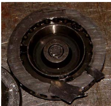
In the first picture we can see where the valve has been smashed and in this case pieces are embedded into the valve plate. The second picture is typical of the damage that is caused when pieces of the valve fall into the cylinder. This type of damage is caused when the compressor tries to pump liquid refrigerant.
