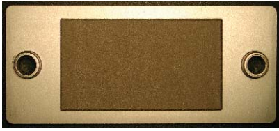
Fig. 9 Demonstrator with a 500µm Ni layer The nickel layer has an area of 47mm to 26mm and a thickness of 500µm and 1000µm. On this sprayed Ni layer the DBC was mounted (42mm to 25mm) in a vacuum soldering process with SnAg3.5 solder. An X-ray analysis (see fig. 10) reveals a few small voids in the solder joint. This is mainly due to the fact, that the solder process parameters have not yet been optimized.
